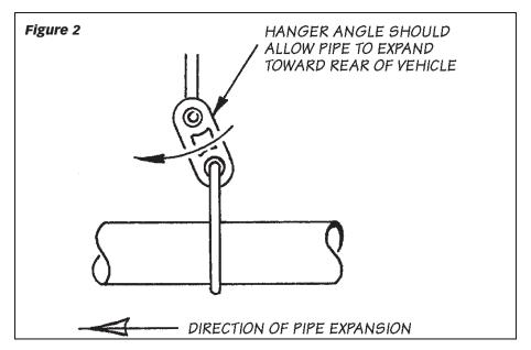
way back. Evenly torque the exhaust clamps to 35 ft-lbs. Make sure that each slip is fully inserted (+/- 1/4 inch).
